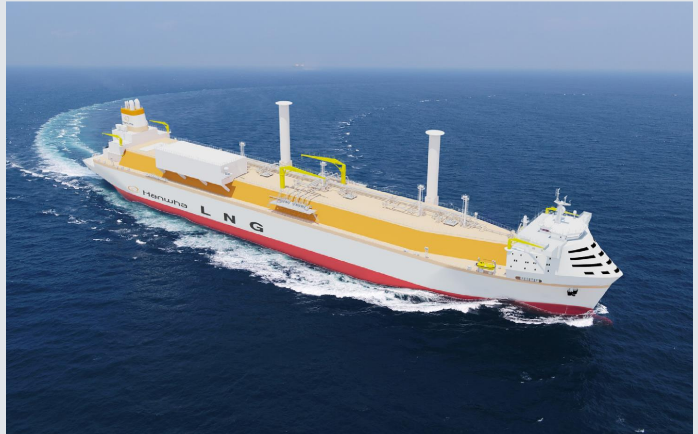
Concept rendering of an LNG carrier powered by an ammonia gas turbine
