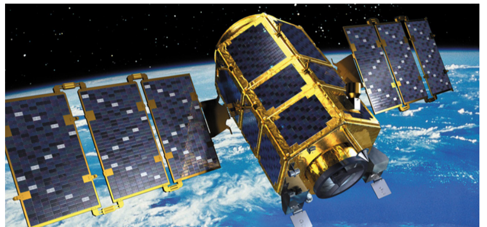
Hanwha Systems provided the infrared sensor system Korea Multi-purpose Satellite (KOMPSAT) 3A uses for nighttime global surveys
