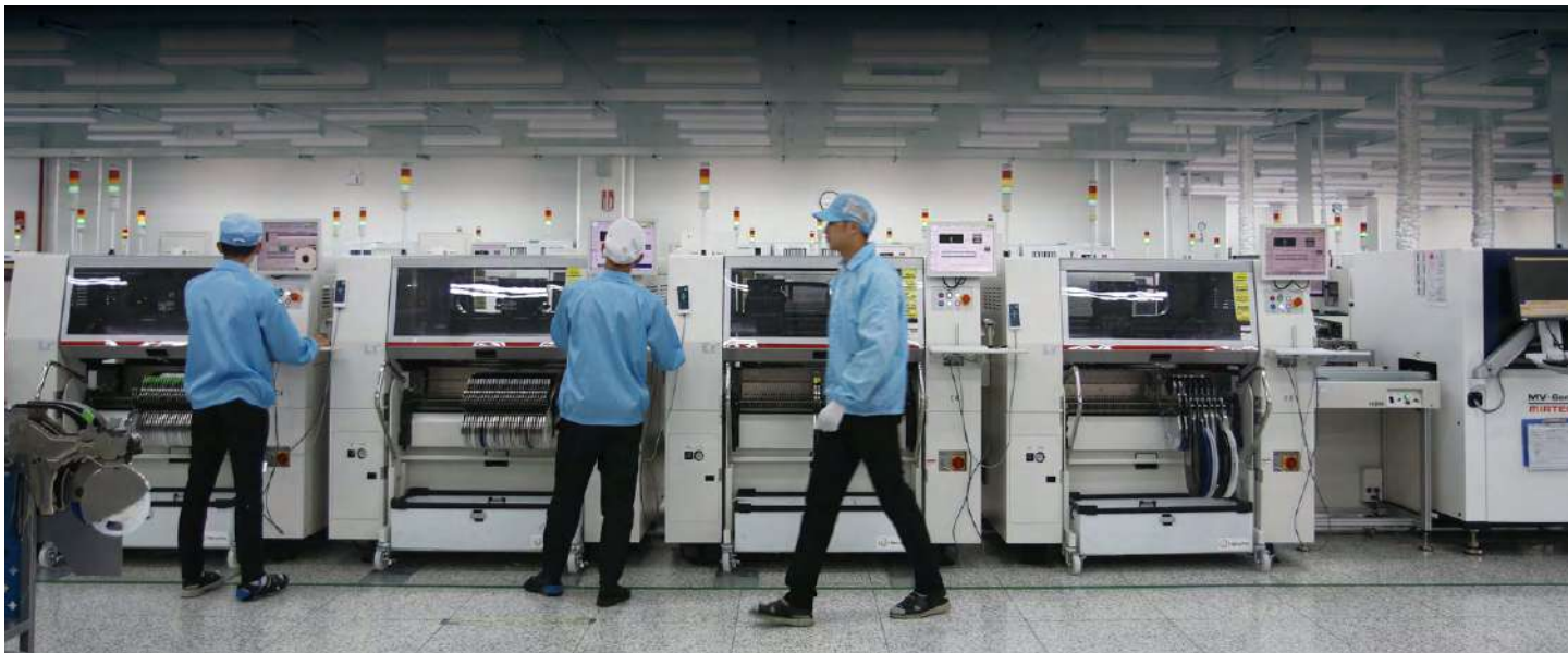
Hanwha Precision Machinery's surface mount technology (SMT) production line
