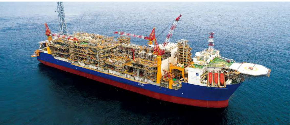
FPSO (Floating Production, Storage, and Offloading)
